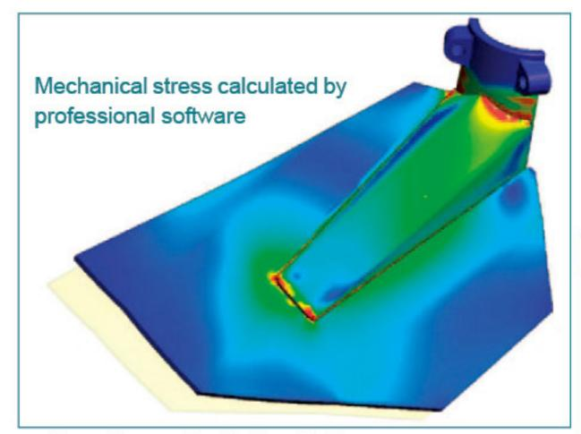
Propeller mechanical analysis
