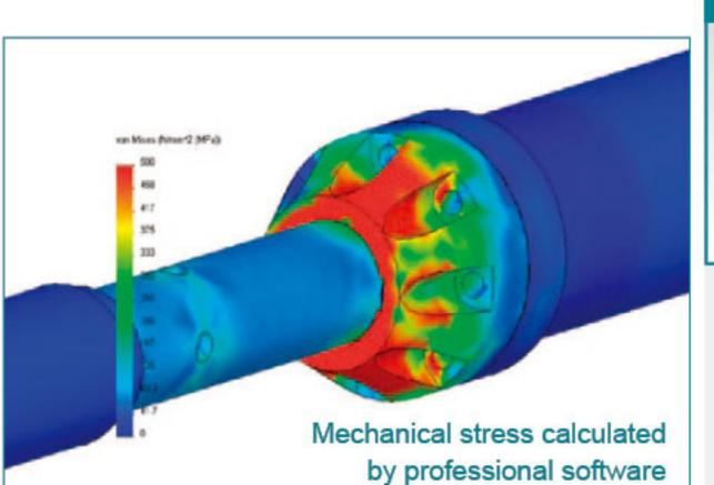
Mechanical analysis of shaft joint
