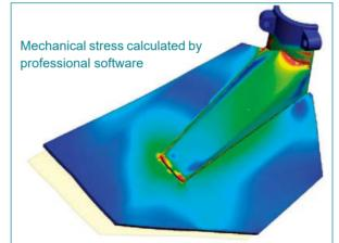
Propeller mechanics analysis
