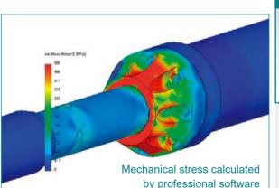
Mechanics analysis of shaft joint
